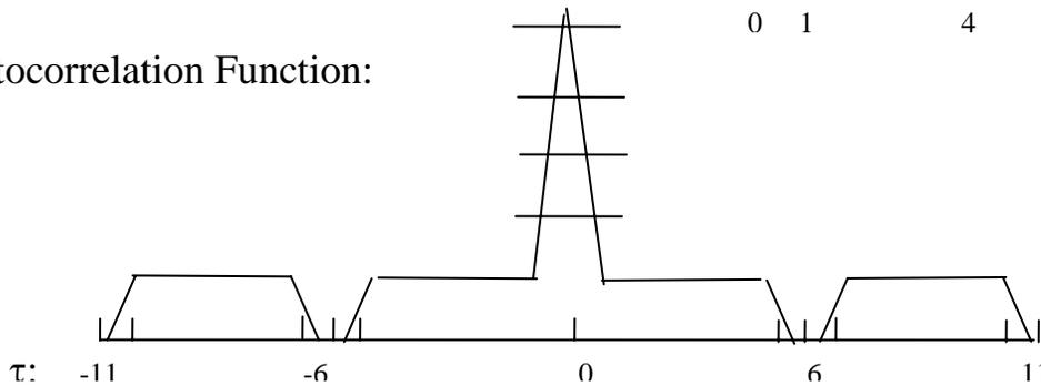
**Figure 51:** The correlation of a radar code pulse train with an image of itself
