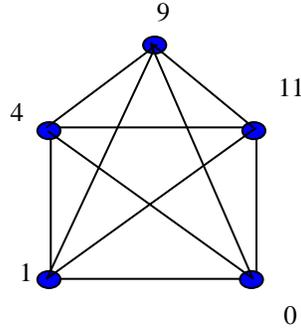
**Figure 50** : Numbering of  $K_5$  with  $\theta(K_5) = 11$
